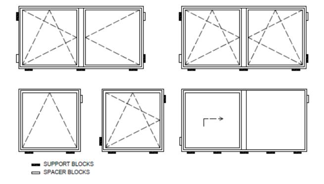
Support and spacer blocks are used to position the window in the opening. Their arrangement varies depending on the type , size of the window and its opening.
