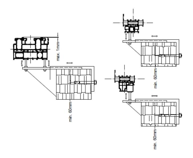
When designing the window fixing, one should also take into account the expansion joint of the building and the structure. The assumed rules in the case of aluminium are the expansion of the profile length of 1000 mm by 1 mm for its cooling in winter and heating in summer. The expansion joint of the structure is provided by special joints of two structures. If, however, it is one structure that exceeds the length of 6000 mm, the expansion joint should be arranged on anchors or mounting brackets.
